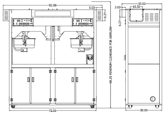
Updraft units need a minimum of 13" clearance on top of unit to change filters.
